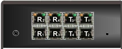
To configure Orion LC for a 4 input, 4 output Cross-Point Switch, set the dip switch 1, 3, and 4 ON and 2 and 5 OFF and connect the CATx or fiber cabling as shown.
