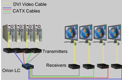
Connect a DVI MM cable from each CPU DVI graphic card to the DVI-In port on the transmitters (1-4)
