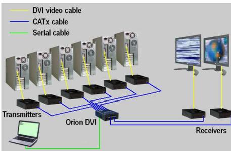
**Figure 10. Cross Point Switch - 6 x 2**
