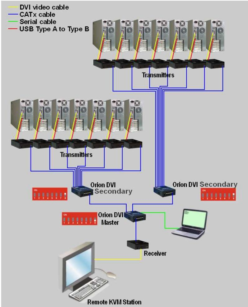
**Figure 15. Single Head KVM Switch (Cascaded)**
