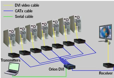
Connect a DVI MM video cable from the CPU's DVI graphic cards to the DVI-In ports on the transmitters.
