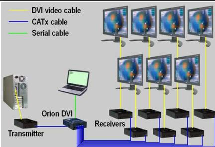
Connect a DVI MM video cable from the CPU's DVI graphic card to the DVI-In port on the transmitter.
