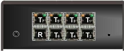
The Single head switch configuration allows you to connect 7 computers to the Orion LC and display and control each computer from a single workstation.
