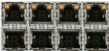
The top row of RJ45 connectors has two LEDs which indicate the LINK status for the top and bottom RJ45 port. The left LED is for the bottom RJ45 port status, the right LED is for the top RJ45 port status.
