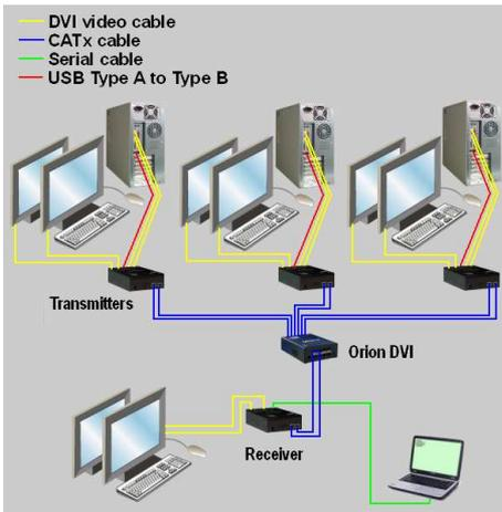
Connect a DVII-MM, a USB Type A to Type B, and optional serial and audio cables to your computer and to the corresponding ports on the transmitter.
