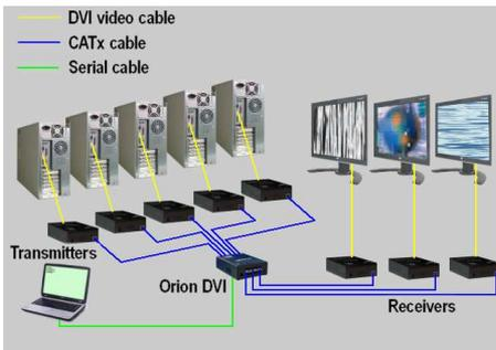
Connect a DVI MM video cable from the CPU's DVI graphic cards to the DVI-In ports on the transmitters.
