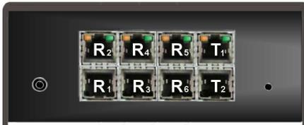
The 2 x 6 configuration allows you to connect 2 computer to the Orion LC and display the video (+audio option) on up to 6 DVI monitors.
