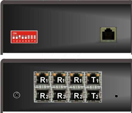
Set the dip switches so that switch 1, 2, 4, and 5 are all in the "OFF" position, switch 3 in the "ON" position.
