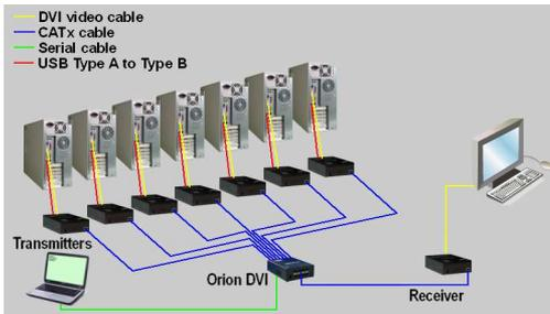
Connect a DVII-MM, a USB Type A to Type B, and optional serial and audio cables to your computer and to the corresponding ports on the transmitter.
