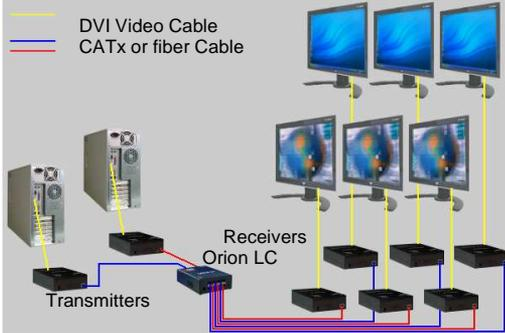
Connect a DVI MM cable from the each CPU DVI graphic card to the DVI-In port on the transmitters
