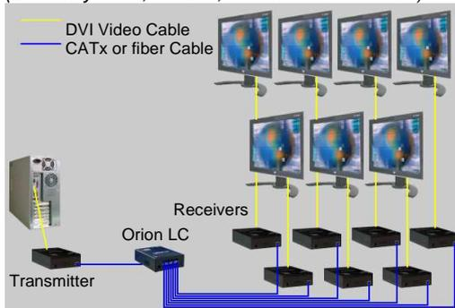
Connect a DVI MM cable from the CPU DVI graphic card to the DVI-In port on the transmitter
