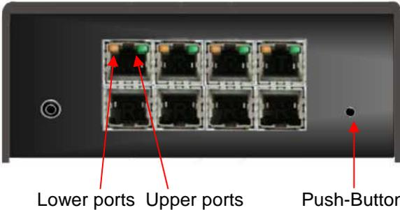
With each press of the push button, the display will switch to the next channel. The channel LED will blink rapidly. When the last channel is reached, the next press will cycle to the first channel.
