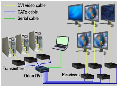
Connect a DVI MM video cable from the CPU's DVI graphic cards to the DVI-In ports on the transmitters.
