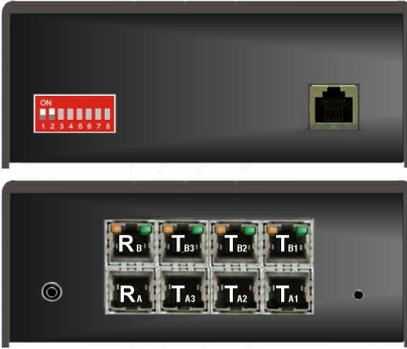
The Dual Head configuration allows you to connect 3 dual video computers to the Orion LC and display and control each computer from a single workstation.
