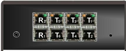
The 6 x 2 configuration allows you to connect 6 computers to the Orion LC and display the video (+audio option) on up to 2 DVI monitors.
