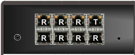
Connector labeled “T” connects to a KVM CATx or fiber transmitter.
