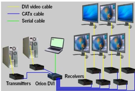
**Figure 6. Cross Point Switch - 2 x 6**
